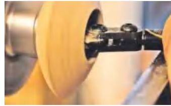
I found addressing the tool too close to horizontal made it drag and catch excessively
